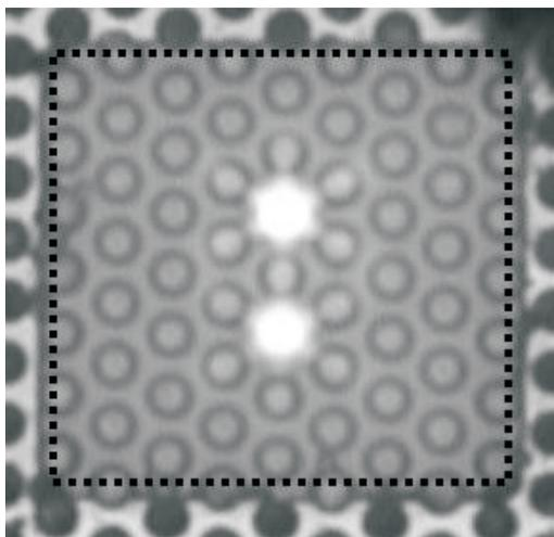
**Fig. 1** Near-field image of photonic crystal VCSEL with two defects lasing in their fundamental modes
