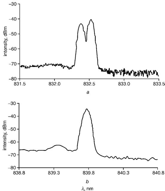
**Fig. 3** Lasing spectra for uncoupled and coupled defects
