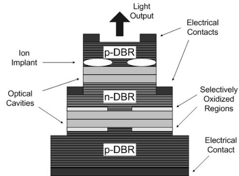
Fig. 1. Device structure of a CRVCL.
