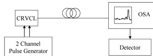
Fig. 4. Setup of CWDM interconnect experiment.
