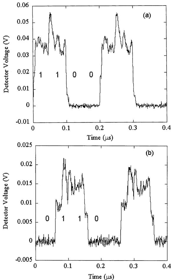
Fig. 6. Logical output from (a) Channel 1 (pattern 1100) and (b) Channel 2 (pattern 0110).
