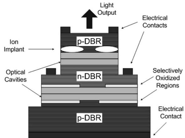
Fig. 1. Device structure for the CRVCL.
