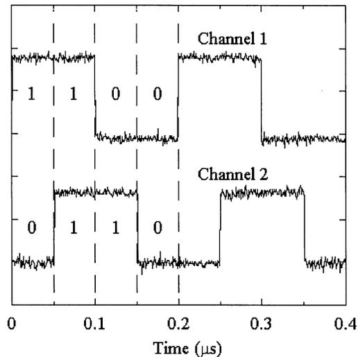
Fig. 5. Electrical inputs to Channel 1 (top) and Channel 2 (bottom) and their corresponding logic values.
