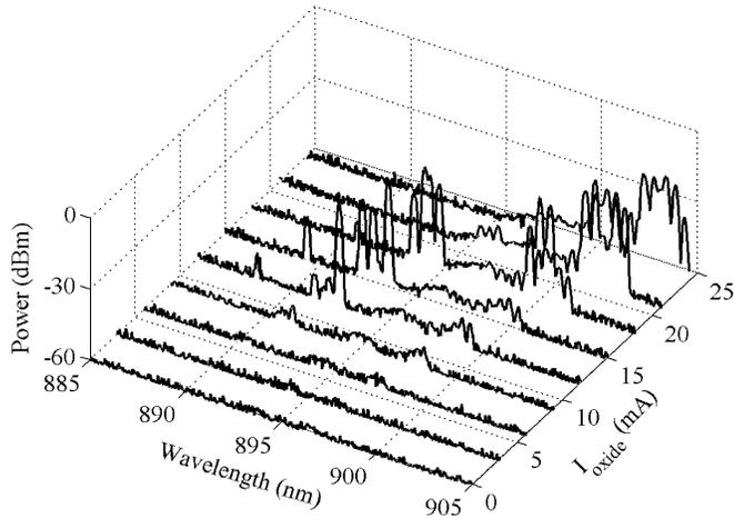
Fig. 2. CRVCL spectra for a constant implant cavity current and varying oxide cavity current.
