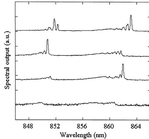
Fig. 3. CRVCL spectral output for the different logic states;  $I_{top}(I_{bottom}) =$ . (a) 0.1 (0.1 mA), (b) 5.1 (0.1 mA), (c) 0.1 (6.1 mA), (d) 5.1 (6.1 mA).
