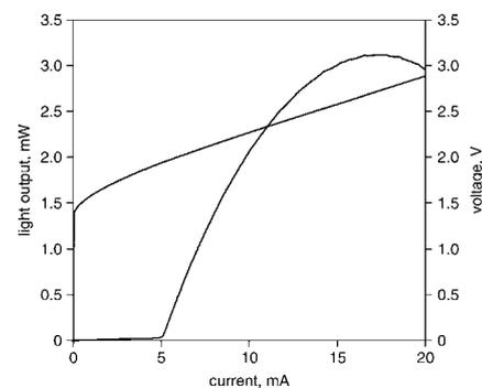
**Fig. 2** Optimised photonic crystal VCSEL with 9  $\mu\text{m}$  oxide aperture operating in single fundamental lateral mode with over 3.1 mW output power
