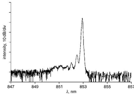
**Fig. 4** Spectral characteristics of optimised singlemode PhC-VCSEL (corresponding to Fig. 2)
