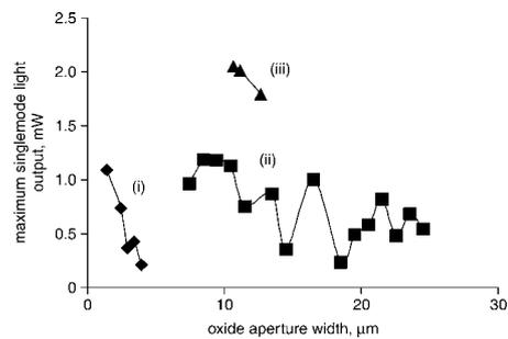
**Fig. 1** Maximum singlemode output power dependence on oxide aperture diameter
