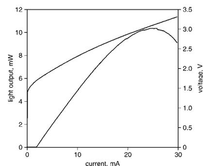
**Fig. 3** Selectively-oxidised VCSEL with 9  $\mu\text{m}$  oxide aperture and no etched holes operating in multiple lateral modes
