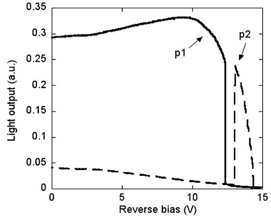
Fig. 5. Polarization-resolved light output from ion-implanted cavity versus reverse bias in oxide-confined cavity.
