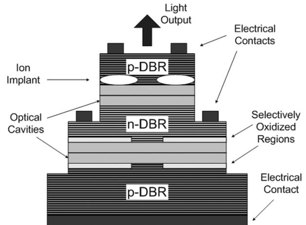
Fig. 1. Device structure for composite-resonator vertical-cavity laser.
