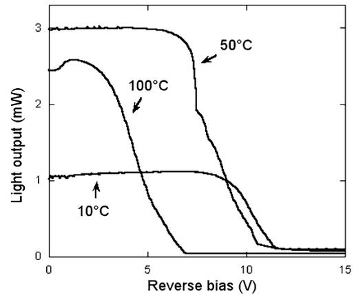
Fig. 9. Unpolarized light output from ion-implanted cavity versus reverse bias in oxide-confined cavity for various temperatures.
