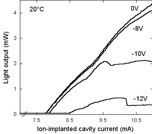
Fig. 2. Unpolarized room-temperature light output characteristics for current sweep in ion-implanted cavity. Oxide-confined cavity biases are labeled on curves.
