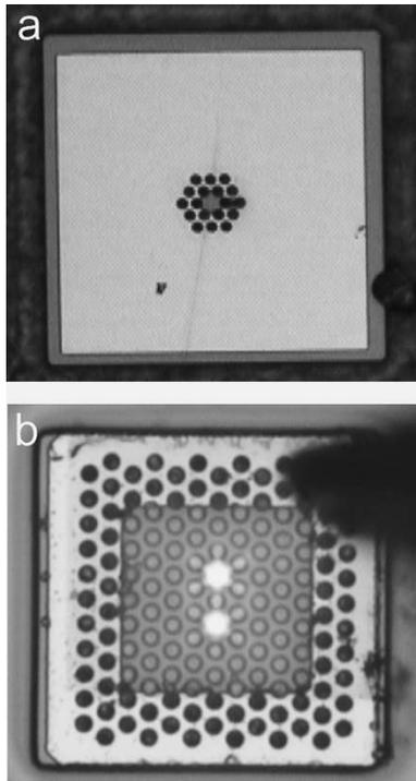
Fig. 3. (a) Photonic crystal pattern created by FIB on an implant VCSEL. (b) Multiple-defect cavity structure patterned by FIB on an oxide VCSEL. FIB enables air holes to perforate a metal contact layer.
