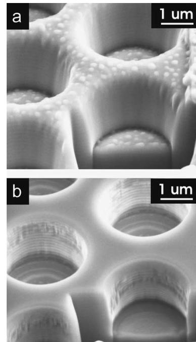
Fig. 2. (a) Holes created by FIB alone show material redeposition, surface roughness, and slightly conical shape. (b) Holes defined by FIB and etched with ICP show negligible surface roughness and are more cylindrical than holes etched with FIB alone. The lower right holes in both SEM images have been milled in cross section.
