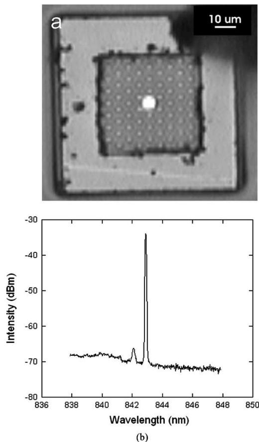
Fig. 5. (a) Near-field pattern of a photonic crystal defect laser in the fundamental mode. (b) Spectrum of the photonic crystal VCSEL.
