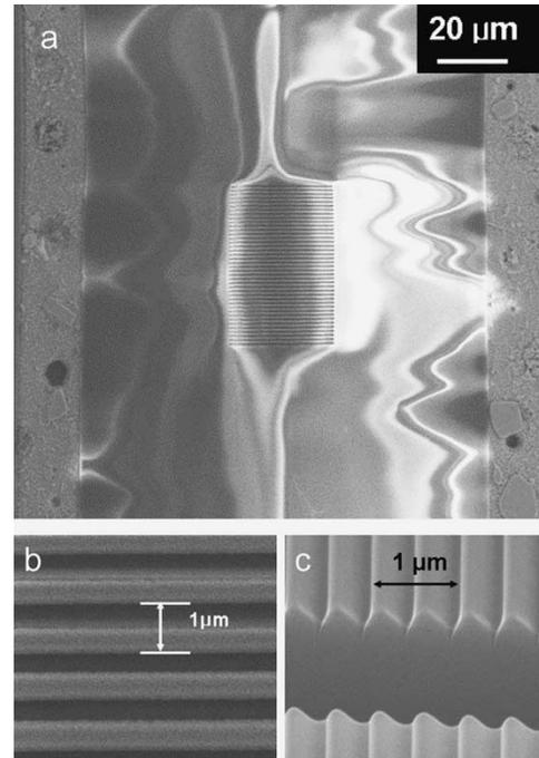
Fig. 4. (a) SEM image of 1D grating created by FIB on a side-polished optical fiber. The bright line in the center corresponds to the 5- $\mu\text{m}$  fiber core. (b) SEM image of 1- $\mu\text{m}$  period gratings. (c) SEM image of 500-nm period gratings and their cross section milled by FIB.
