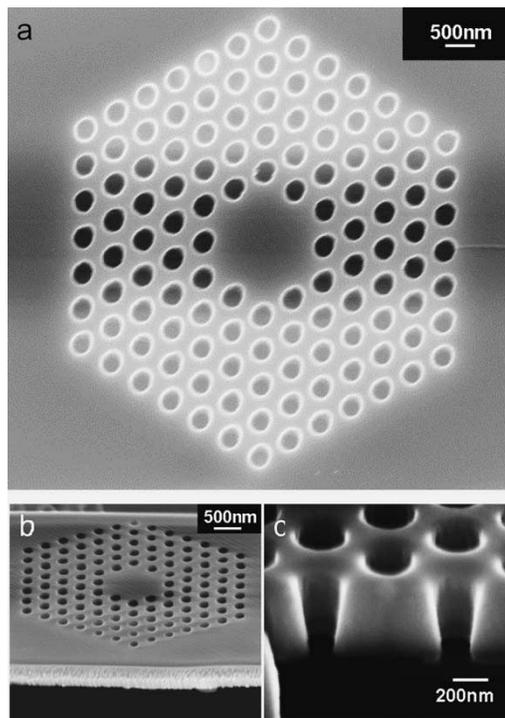
Fig. 6. (a) SEM image of a photonic crystal defect cavity structure defined by FIB. (b)  $60^\circ$  perspective SEM image of an undercut etched sample. (c) FIB milled cross section SEM image of an undercut etched sample.
