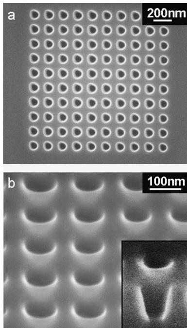
Fig. 1. (a) SEM image of  $10 \times 10$  array holes patterned by FIB with ion beam current of 50 pA. (b)  $52^\circ$  perspective SEM image of the array pattern. The lower right inset shows the cross section milled by FIB. The measured depth of the hole is 125 nm.
