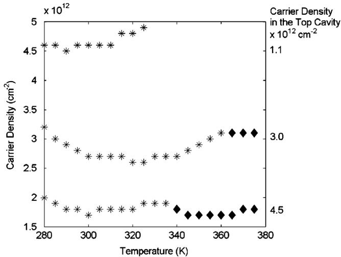
Fig. 8. Modeled threshold carrier density of the top cavity and dominant longitudinal mode for various biases on the bottom cavity. An asterisk indicates that the short wavelength lased, and a diamond indicates that the long wavelength lased. Threshold gain is assumed to be at  $1500 \text{ cm}^{-1}$ .
