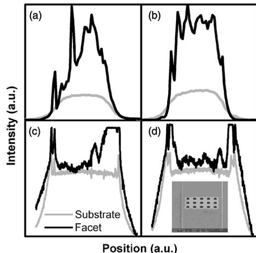
FIG. 1. Measured emission profiles at  $0.5I_{th}$  (gray lines) and  $8I_{th}$  (black lines) from 150  $\mu\text{m}$  stripe broad area lasers with and without  $p$ -side patterning. The inset of (d) shows the pattern. (a) Near field (unpatterned sample). (b) Near field (patterned sample). (c) Spontaneous emission from substrate (unpatterned). (d) Spontaneous emission from substrate (patterned).
