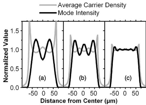
FIG. 2. Theoretical optical intensity and average carrier density profiles for structures with optical profile defined by (a) two, (b) three, and (c) six transverse optical modes at a current of  $8I_{th}$ .
