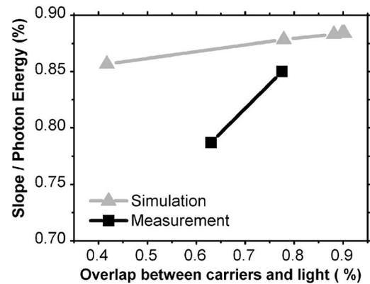
FIG. 3. Normalized slope as function of overlap between optical mode and carrier density—experimental and theoretical.
