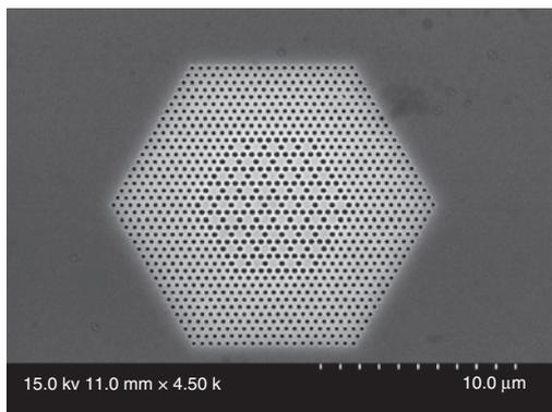
**Fig. 1** Image of photonic crystal heterostructure laser cavity
