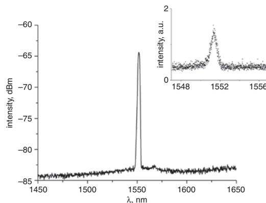
**Fig. 3** Lasing spectrum at pump power of 13 mW
