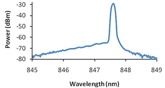
Fig. 9. Optical spectrum of a single-mode, two-by-one implanted VCSEL array.
