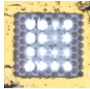
Fig. 13. Near-field image of a four-by-four photonic crystal VCSEL array.
