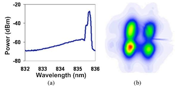
Fig. 14. (a) Optical spectrum and (b) out-of-phase far-field intensity of the four-by-four photonic crystal VCSEL array.
