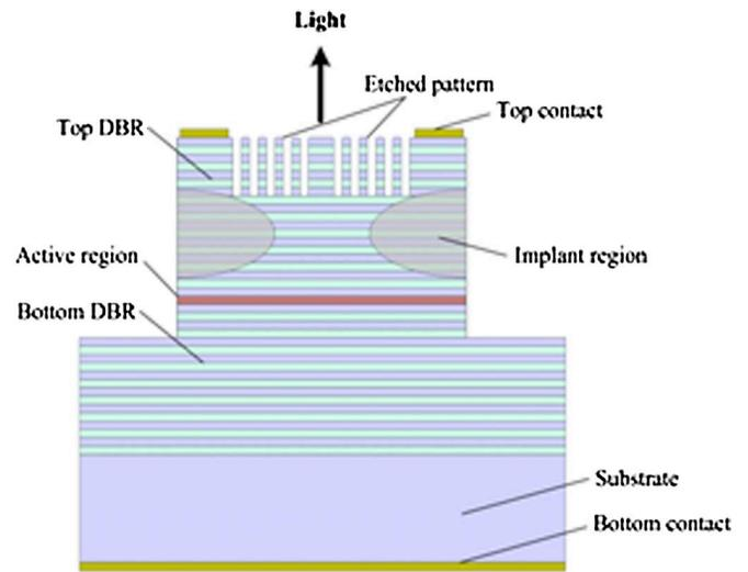
Fig. 1. Cross-sectional sketch of a photonic crystal VCSEL.
