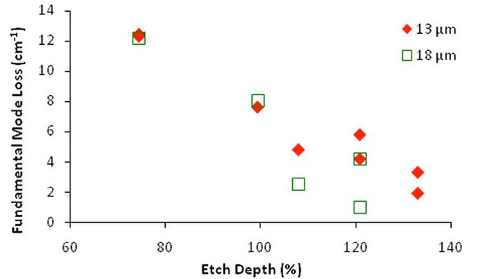
Fig. 6. Plot of the calculated fundamental mode loss against the measured etch depth in percent depth through the top DBR for single-mode photonic crystal VCSELs with  $a = 4.0 \mu\text{m}$  and  $b/a = 0.7$ .
