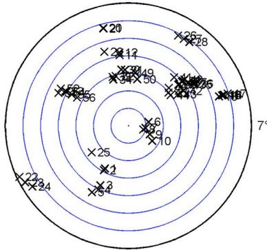
Fig. 12. Map of the angular location of the far-field intensity maximum for different current injection schemes into a three-element array.
