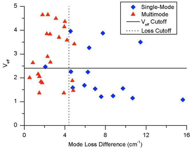
Fig. 5. Plot of the  $V_{\text{eff}}$  parameter against the difference in loss between the fundamental and first higher order modes. The single-mode  $V_{\text{eff}}$  cutoff is shown as a solid line and the apparent loss discrimination cutoff is shown as a dotted line.
