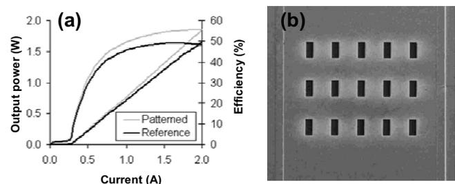
FIG. 1. (a) Light-current-efficiency characteristics of the etched and unetched reference broad area semiconductor lasers. (b) SEM image of the FIB-etched hole pattern in the laser stripe.
