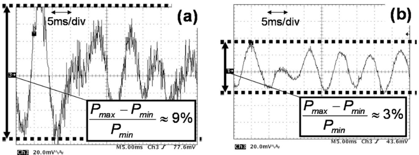
FIG. 3. Measured photodetector waveforms for the unpatterned broad area semiconductor laser (a) without and (b) with etched holes measured through an effective 7  $\mu\text{m}$  aperture. The data are taken at the same current injection level, with the dc component of the signal removed for illustration purposes.
