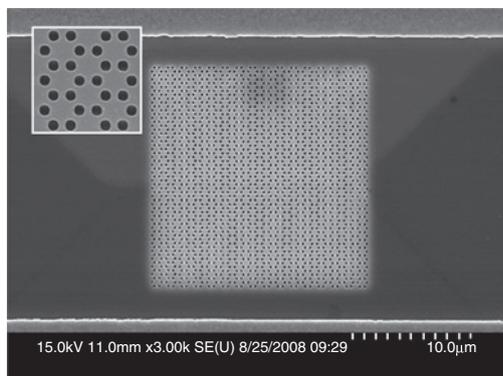
Fig. 2 SEM image of LCI graphene PhC with metal contacts; also visible are doped regions of diode
