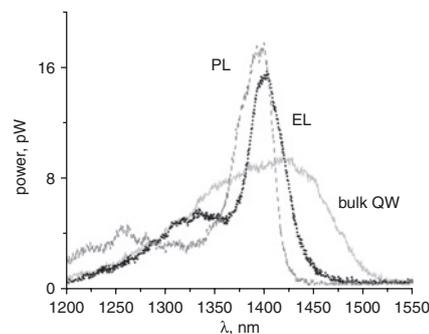
Fig. 3 Emission spectra of LCI PhC: EL from an unpatterned quantum well, EL from the PhC, and PL from the PhC
