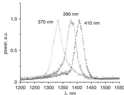
Fig. 4 Resonance tuning of EL spectra from graphene PhCs with differing lattice constants
