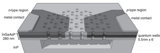
Fig. 1 Schematic of LCI PhC emitter, shown in cross-section
