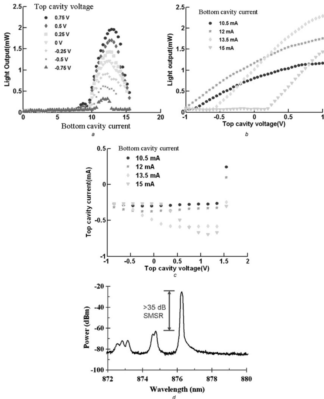
**Figure 2** CW characteristics of the CRVCL using on-wafer probing at room temperature
