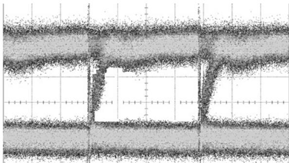
**Figure 5** Large-signal modulation eye diagram (unfiltered) taken at 54 Mbps
