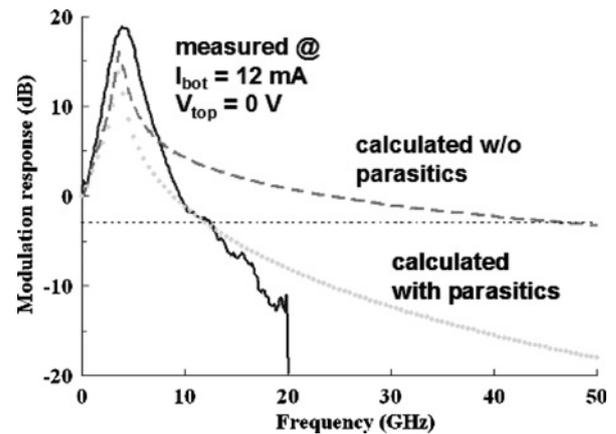
**Figure 4** Calculated modulation response of a CRVCL under intracavity electroabsorption modulation without parasitic effects (solid curve) and with parasitic effects (dashed curve)
