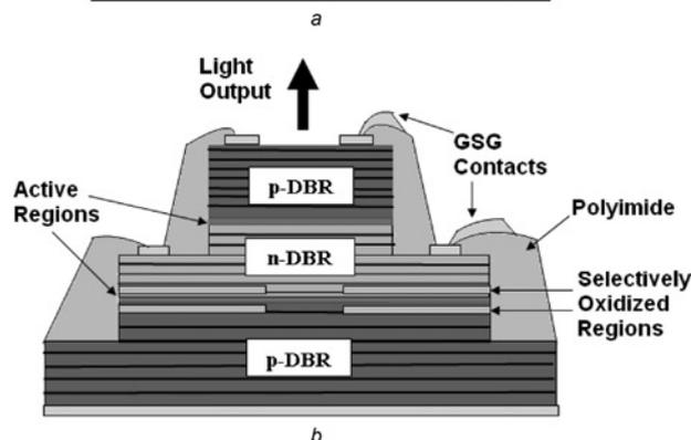
**Figure 1** Device cross-section and image of the scanning electron microscope
