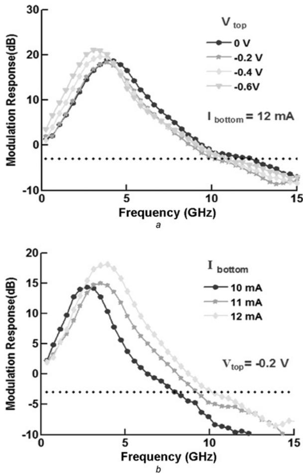
**Figure 3** Small-signal modulation response of the CRVCL at different dc voltage biases
