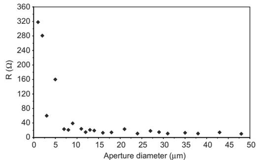
**Fig. 6.** Variation of differential series resistance with aperture size.
