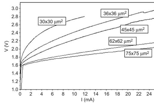
Fig. 5.  $I-V$  characteristics of fabricated VCSEL devices with various mesa sizes.
