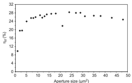
**Fig. 10.** Plot of differential quantum efficiency with various oxide apertures.
