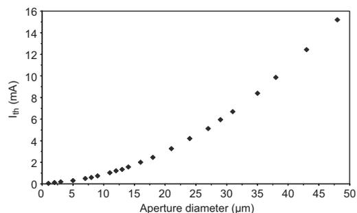
**Fig. 8.** Variation of threshold current with aperture size for fabricated VCSELs.
