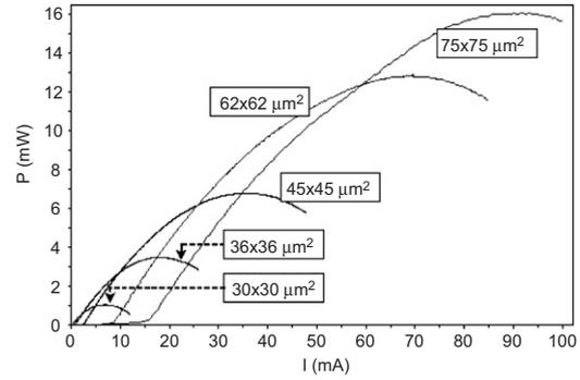
Fig. 4.  $L-I$  characteristics of fabricated VCSEL devices with various mesa sizes.
