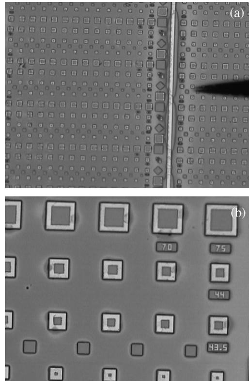
Fig. 2. (a) Various fabricated 850 nm VCSEL devices; (b) larger view of VCSEL mesa sizes.
