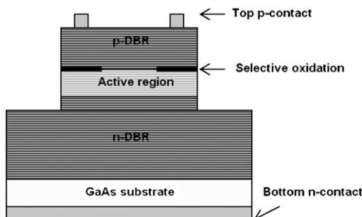
Fig. 1. Schematic of 850 nm VCSEL device.
