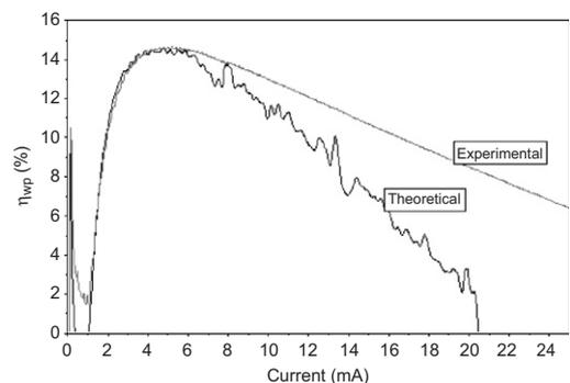
**Fig. 11.** Plot of wall-plug efficiency with input current for a VCSEL with  $11 \times 11 \mu\text{m}^2$  oxide aperture size.
