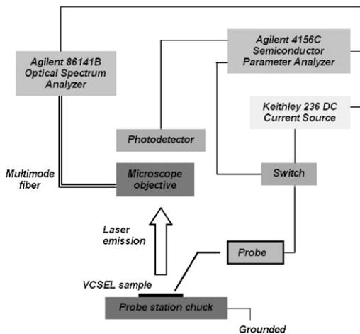
Fig. 3. The experimental measurement setup.
