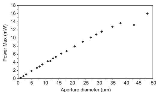
**Fig. 7.** Variation of maximum output power with aperture size.
