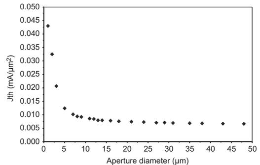
**Fig. 9.** Variation of threshold current density with aperture size.
