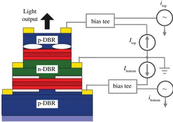
Fig. 1. Schematic of the CRVCL device structure.
