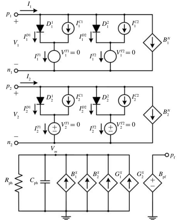
Fig. 3. Circuit-level implementation to model the CRVCL.
