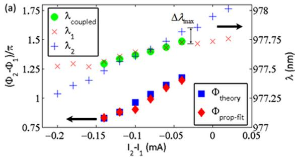
FIG. 5. Measured peak wavelength values and native resonances retrieved within the locking range. Propagated-fit phase measurements are also compared to that calculated from Eq. (6).
