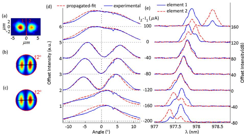
FIG. 4. (a) Near field amplitude, (b) propagated-fit, and (c) experimentally determined far-field intensity images for  $I_1 = 3.6\ \text{mA}$ . (d) Far field profiles are taken across the lines shown in (b) and (c) and are compared under varying differential current injection. (e) Corresponding spectra captured from elements 1 and 2, as delineated in (a).
