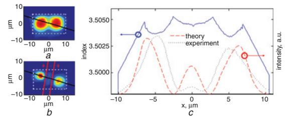
Fig. 3 Near-field intensities and refractive index for  $2 \times 1$  array
