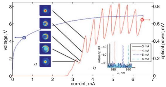
Fig. 2 Output characteristics for single,  $5 \mu\text{m}$  diameter VCSEL
