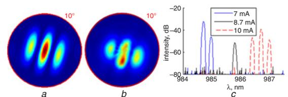
Fig. 4 Far-field intensities and spectral data for  $2 \times 1$  array
