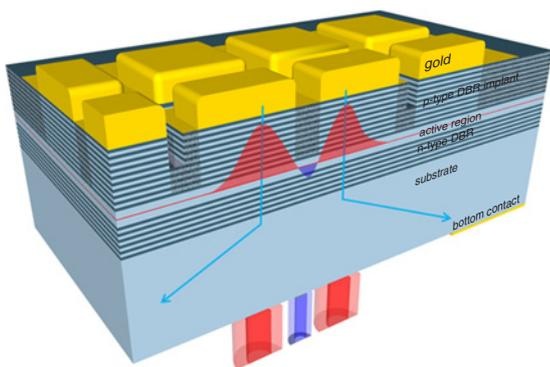
Fig. 1 Bottom-emitting 2D VCSEL array structure
