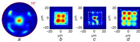
**Fig. 5** Near- and far-field intensities from  $2 \times 2$  and  $3 \times 3$  arrays
