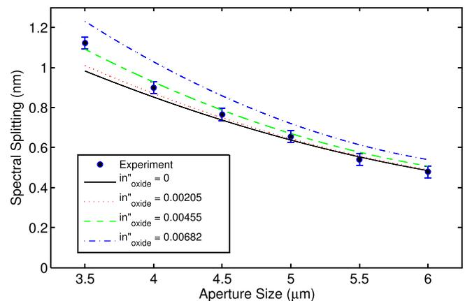
FIG. 2. Plot of measured subthreshold spectral splitting between fundamental and first higher-order mode as function of aperture size with error bars corresponding to the  $0.06 \text{ nm}$  resolution of the optical spectrum analyzer. The curves are calculated from Eq. (4), for varying values of  $n''_{oxide}$  equal to 0, 5, 10, and  $15 \text{ cm}^{-1}$  for the  $3.5 \mu\text{m}$  aperture VCSEL.
