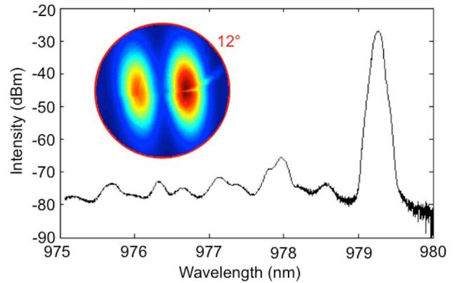
Fig. 5. Spectra of coherently coupled  $2 \times 1$  VCSEL array under direct modulation giving bandwidth enhancement. The corresponding far-field intensity image inset shows out-of-phase coherent coupling.
