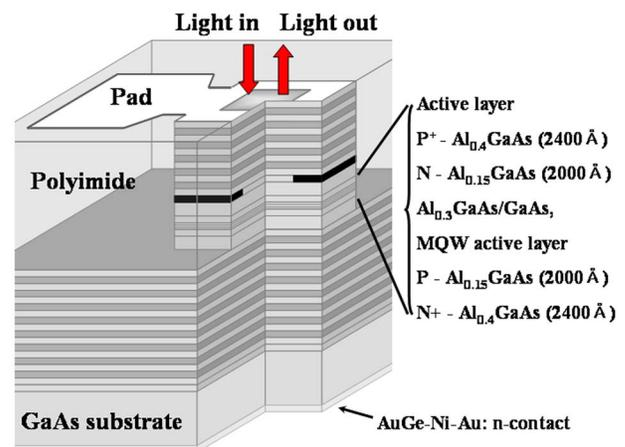
FIG. 1. Cross section of the oxidized vertical cavity laser with the depleted optical thyristor structure.
