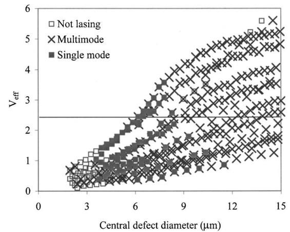
FIG. 3. Comparison of calculated and observed modal properties of photonic crystal VCSELs vs defect diameter.
