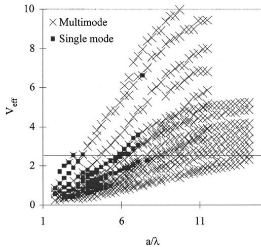
FIG. 2. Comparison of calculated and observed modal properties of photonic crystal VCSELs with lattice constant  $a$ . Devices are positioned onto the plot with the theoretical model and the actual operation is depicted by the data points.
