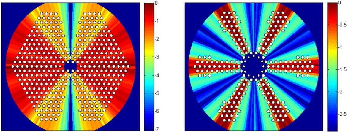
Fig. 1. Depiction of the algorithm used to help determine which holes are removed in a decimated design for (a) L3 ( $a = 370$  nm) and (b) H2 ( $a = 450$  nm) cavities. The summed field intensities in each sector are on a log scale.
