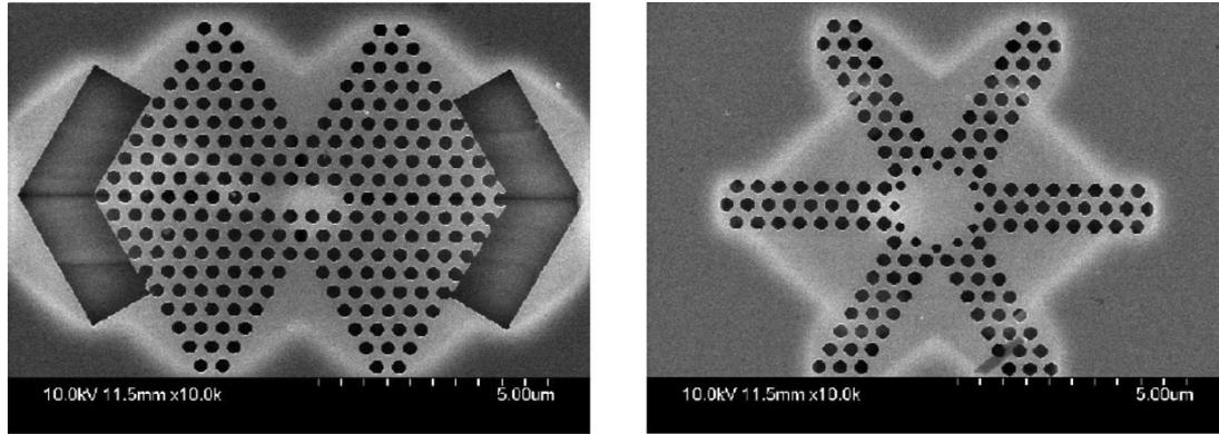
Fig. 4. (a) Fabricated decimated L3 and (b) H2 photonic crystal defect cavity lasers.
