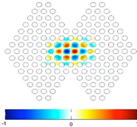
Fig. 2. Modal profile (magnetic field component) of decimated L3 photonic crystal defect cavity ( $a = 470$  nm) determined by 3-D FDTD calculation.
