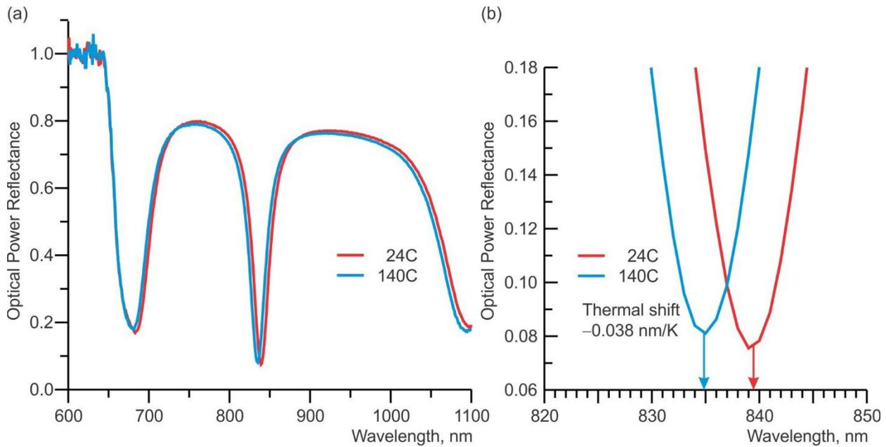
Fig.8. Optical power reflectance spectra of a resonant  $\text{SiO}_2/\text{Ta}_2\text{O}_5$  structure with a  $\lambda/2$   $\text{SiO}_2$  resonant cavity. (a) coarse scale. (b) fine scale showing the shift of the reflectivity dip.
