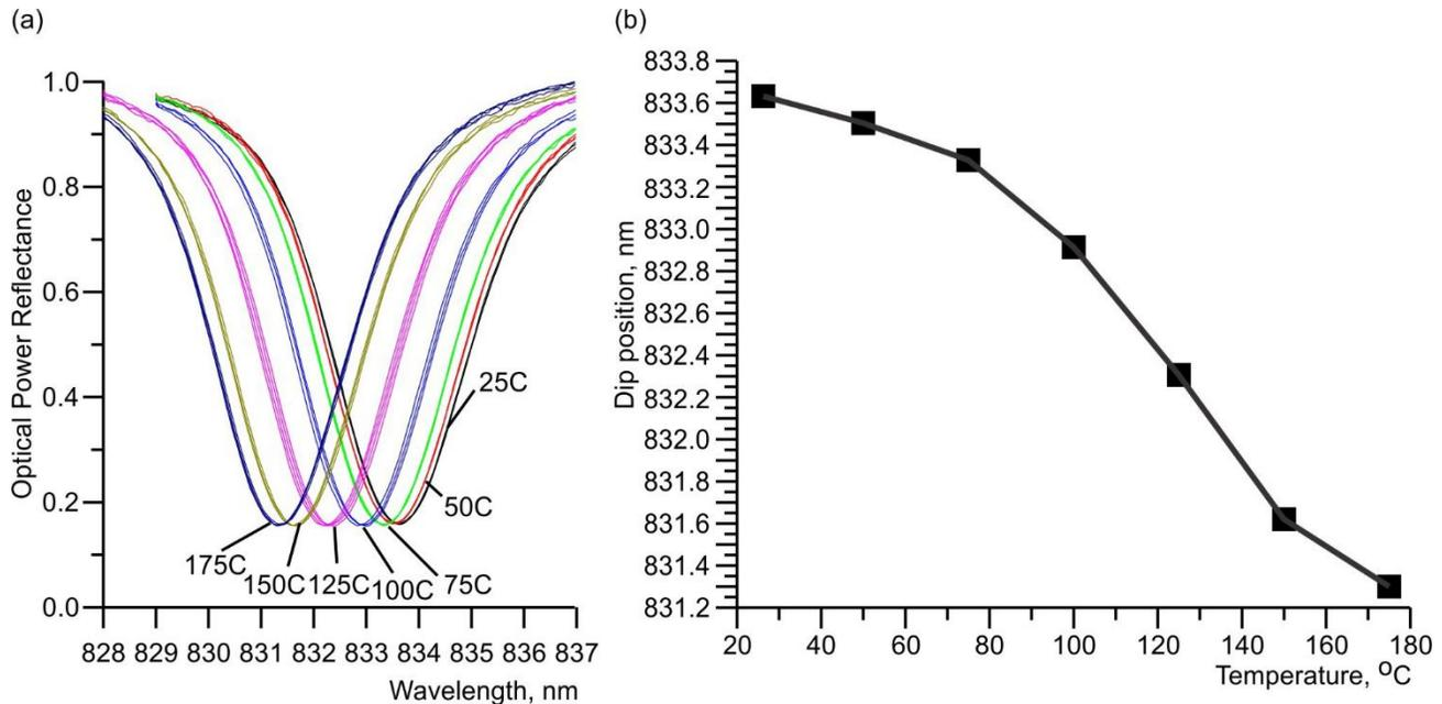
Fig.5 (a) Optical power reflectance spectra of Structure #2 of Fig. 1 containing TiO<sub>2</sub> cavity in the vicinity of the reflectivity dip at various temperatures. (b) Temperature shift of the dip position.
