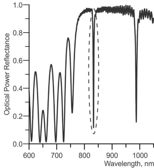
Fig.4 Optical power reflectance spectrum of the structure #2 of Fig. 1 containing TiO<sub>2</sub> cavity.
