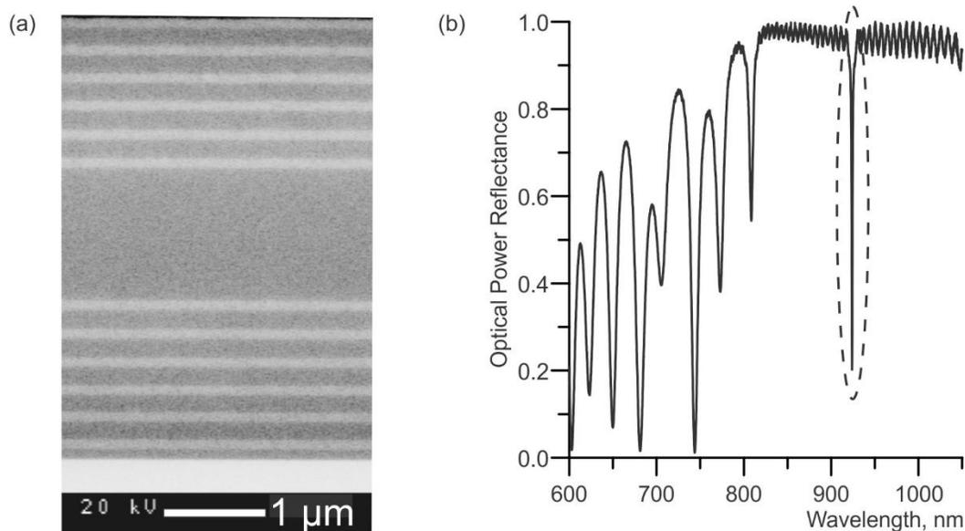
Fig.2. (a) Cross-sectional scanning electron microscopy image of the test resonance structure #1 of Fig. 1 containing SiO<sub>2</sub> cavity. (b) Optical power reflectance spectrum of the structure #1.
