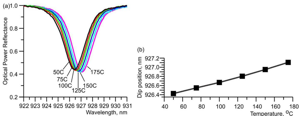
Fig.3. (a) Optical power reflectance spectra of Structure #1 of Fig. 1 containing SiO<sub>2</sub> cavity in the vicinity of the reflectivity dip at various temperatures. (b) Temperature shift of the dip position.
