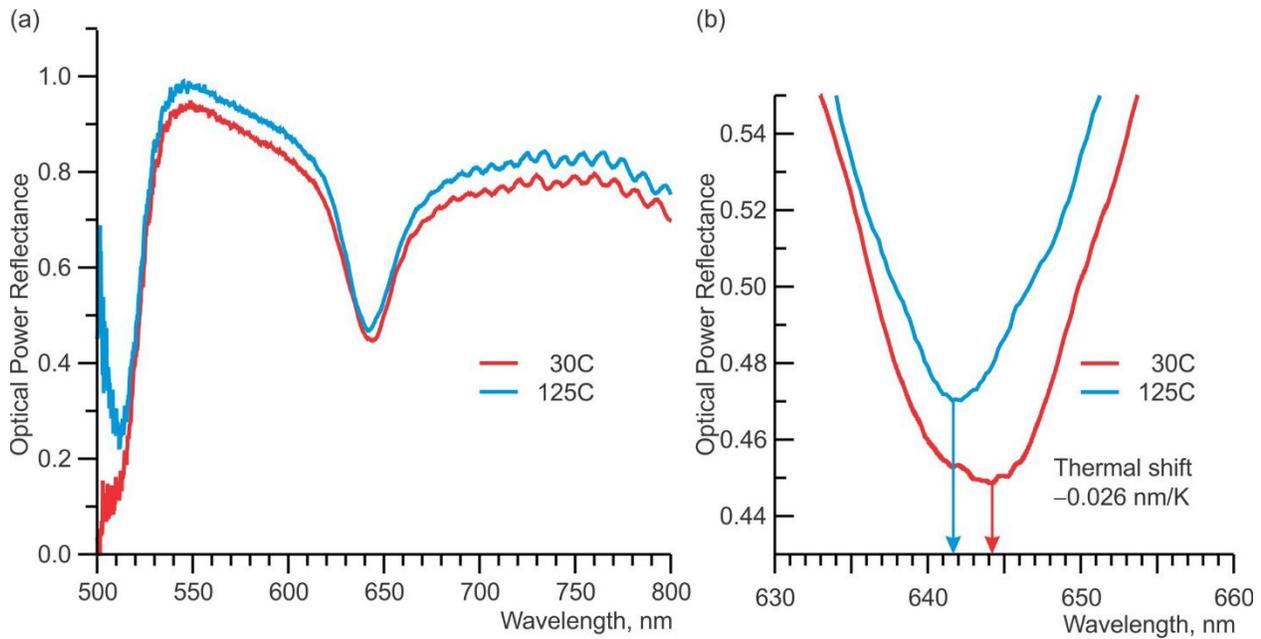
Fig.9. Optical power reflectance spectra of a resonant  $\text{SiO}_2/\text{Ta}_2\text{O}_5$  structure with a  $\lambda/2$   $\text{SiO}_2$  resonant cavity designed for 650 nm spectral range. (a) coarse scale. (b) fine scale showing the shift of the reflectivity dip.
