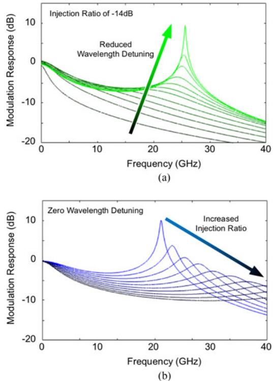
Fig. 3. Simulated modulation response curves for (a) decreasing value of wavelength or phase detuning at a fixed injection ratio and (b) increasing injection ratio at a fixed wavelength detuning of zero, for one element being injection locked by another.
