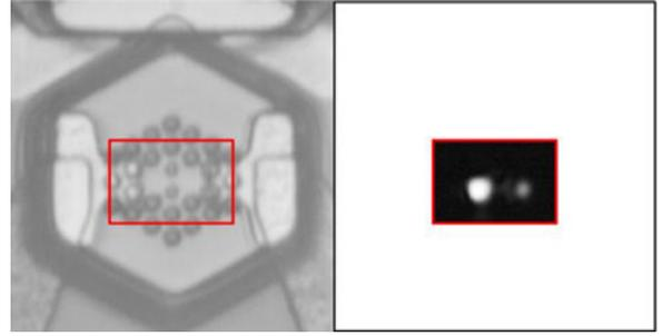
Fig. 7. Micrographs of (left) hexagonal-lattice VCSEL array with  $b = 2.7$   $\mu\text{m}$  and  $b/a = 0.6$  and (right) near-field intensity with the left element having  $I_1 = 7.9$  mA and the right element having  $I_2 = 6.8$  mA and small signal modulation applied.
