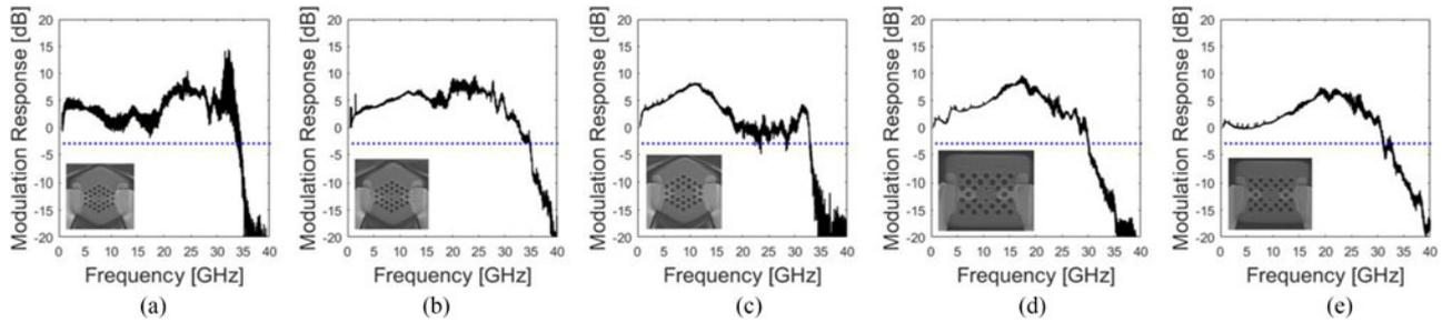
Fig. 9. Small signal modulation response showing 3-dB bandwidth beyond 30 GHz for devices with each of five photonic crystal designs on sample. A scanning electron micrograph of the corresponding device is shown by the inset.
