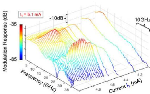
Fig. 6. Modulation response vs. bias currents ( $I_1 = 5.1$  mA while  $I_2$  is varied) throughout the locking range.
