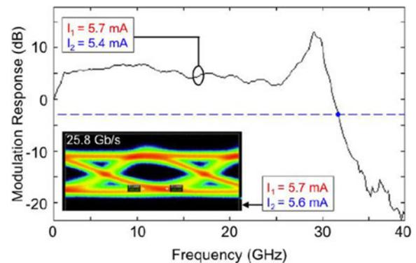
Fig. 10. Small signal response and inset eye-diagram showing open eyes at 25 Gb/s data rate.
