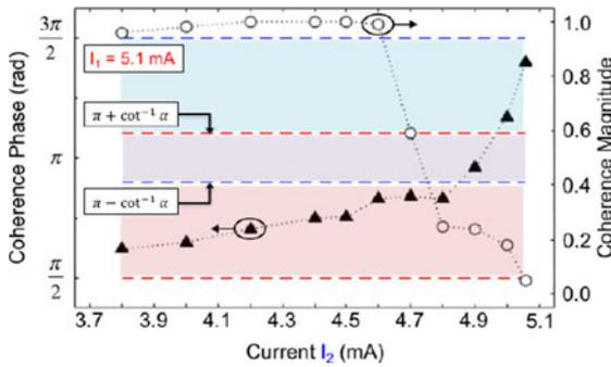
Fig. 5. Coherence phase (triangle) and magnitude (circle) extracted via near- and far-field analysis. Phase constraints of injection locking for Element 1 and Element 2 are indicated with red and blue, respectively, dashed lines and shading.
