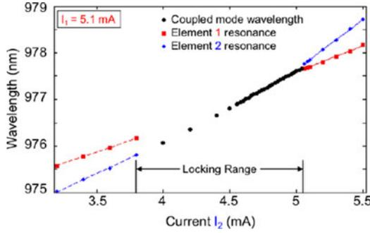
Fig. 4. Spectral data showing resonance wavelength vs. bias currents ( $I_1 = 5.1$  mA while  $I_2$  is varied) for fundamental modes of elements 1 (red square) and 2 (blue diamond) and the coupled mode (black circles) through locking range.
