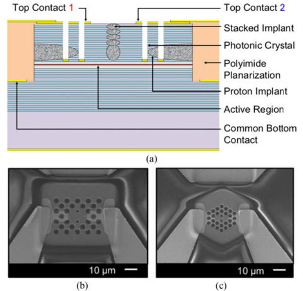
Fig. 1. (a) Cross-sectional sketch and (b) and (c) scanning electron micrographs of  $1 \times 2$  optically coupled, phased vertical cavity laser array. The array in (b) has square-lattice with  $b = 3.6 \mu\text{m}$  and  $b/a = 0.6$  and the array in (c) has hexagonal-lattice with  $b = 2.4 \mu\text{m}$  and  $b/a = 0.6$ .
