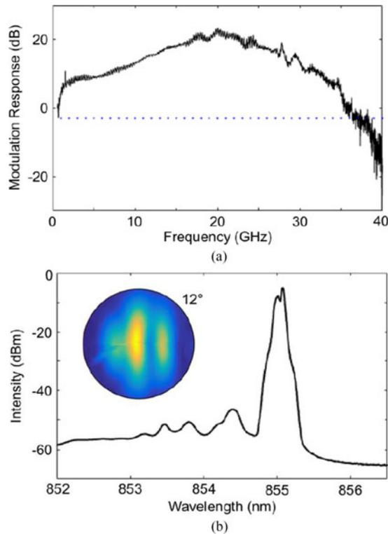
Fig. 11. (a) Small signal modulation response and (b) optical spectrum with inset far-field intensity profile for  $1 \times 2$  phased VCSEL array (hexagonal lattice with  $b = 2.7 \mu\text{m}$  and  $b/a = 0.6$ ) with small signal modulation applied to Element 2 and DC bias of  $I_1 = 7.2 \text{ mA}$  and  $I_2 = 7.1 \text{ mA}$ .
