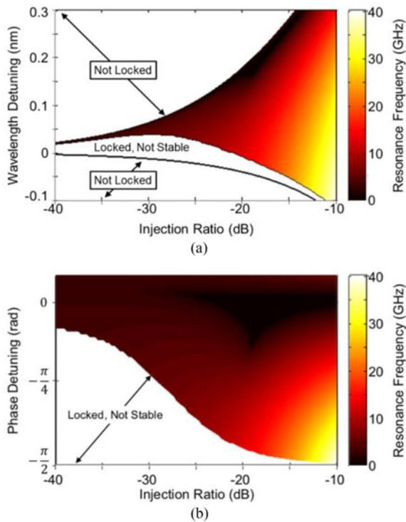
Fig. 2. Simulated maps of the locking range showing modulation response resonance frequency vs. injection ratio and (a) spectral resonance wavelength detuning or (b) relative coupling phase detuning for one element being injection locked by another.
