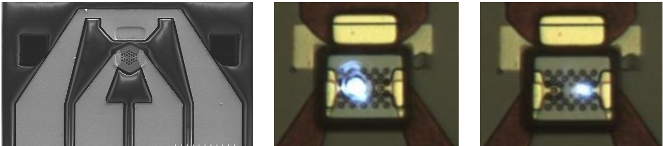
Figure 1: 2 \times 1 photonic crystal VCSEL arrays (left is SEM image, center and right are microscope photographs with either the left or right cavity lasing).
